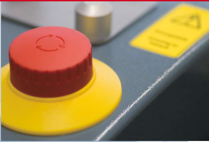
Emergency off switch
