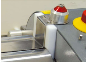
Protection coverings at the roller shafts
