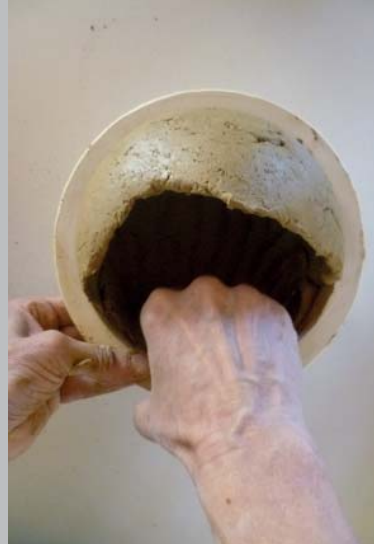
The formed hemisphere is thrown a part out of the mould...
