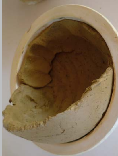
Forming an object from the body, e.g. a ball from a hemisphere plaster mould.
