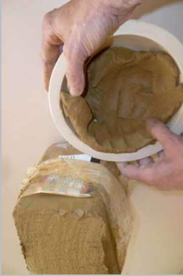
Forming an object from the body, e.g. a ball from a hemisphere plaster mould.
