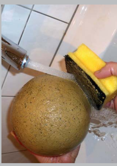
The leather hard body is finished under running water with a brush...
