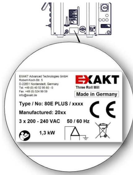
Fig. 3: Type plate of the machine 200-240V – Corner grounded Delta
